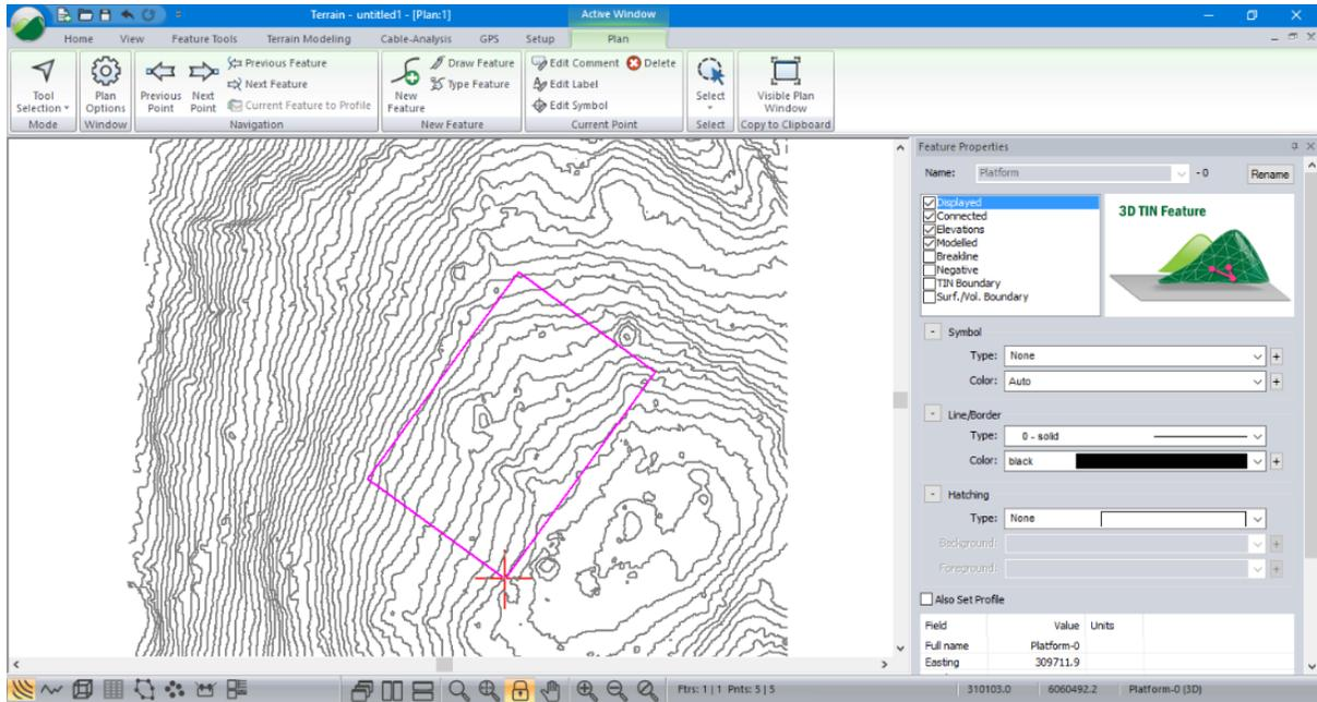
Figure 10-4: Initial Pad Location Overlaid on Topo Contours
