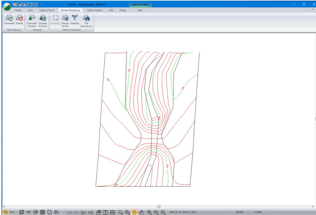
Figure 8-14: Model of Creek with Poorly Generated Contours
