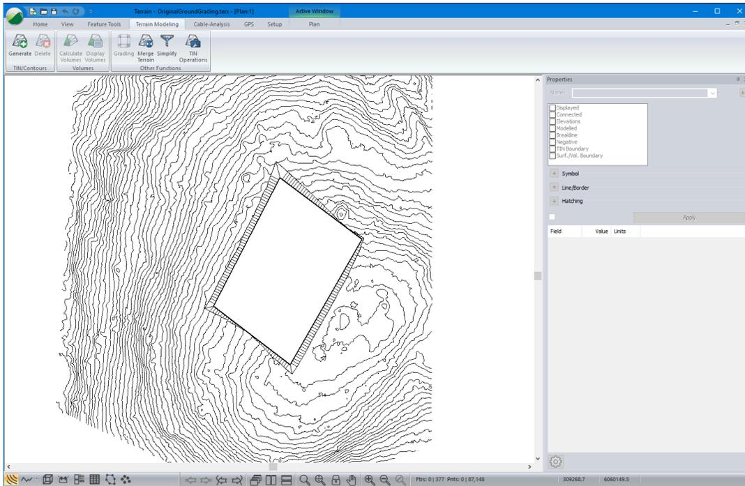
Figure 10-17: Platform Merged into OriginalGroundGrading.terx
