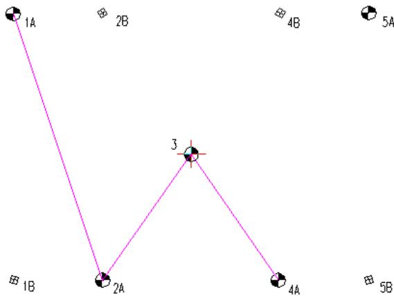
Figure 3-6: Inserting a Point at the Middle of a Segment
