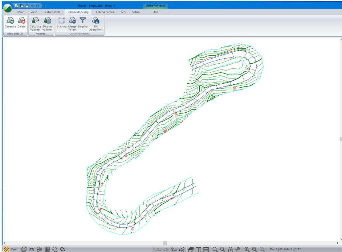
Figure 8-8: Contours Generated with Side Length Control
