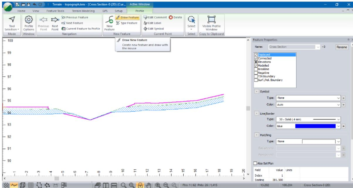
Figure 9-10: Profile Window with Multiple Layers
