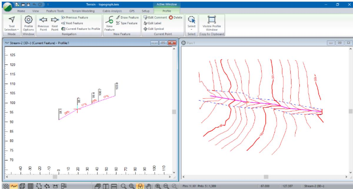
Figure 9-4: Stream Profile with Elevations and Grades
