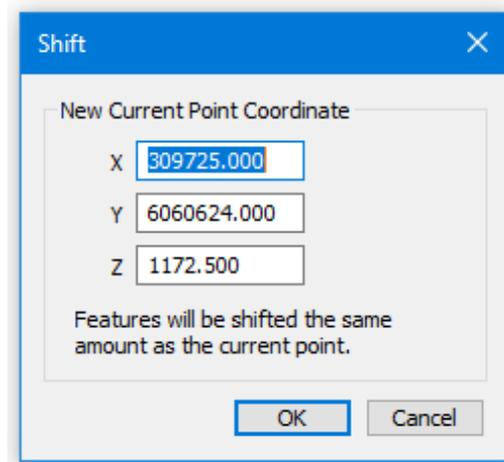
Figure.10-12: Using Shift to change elevation of “Platform”
