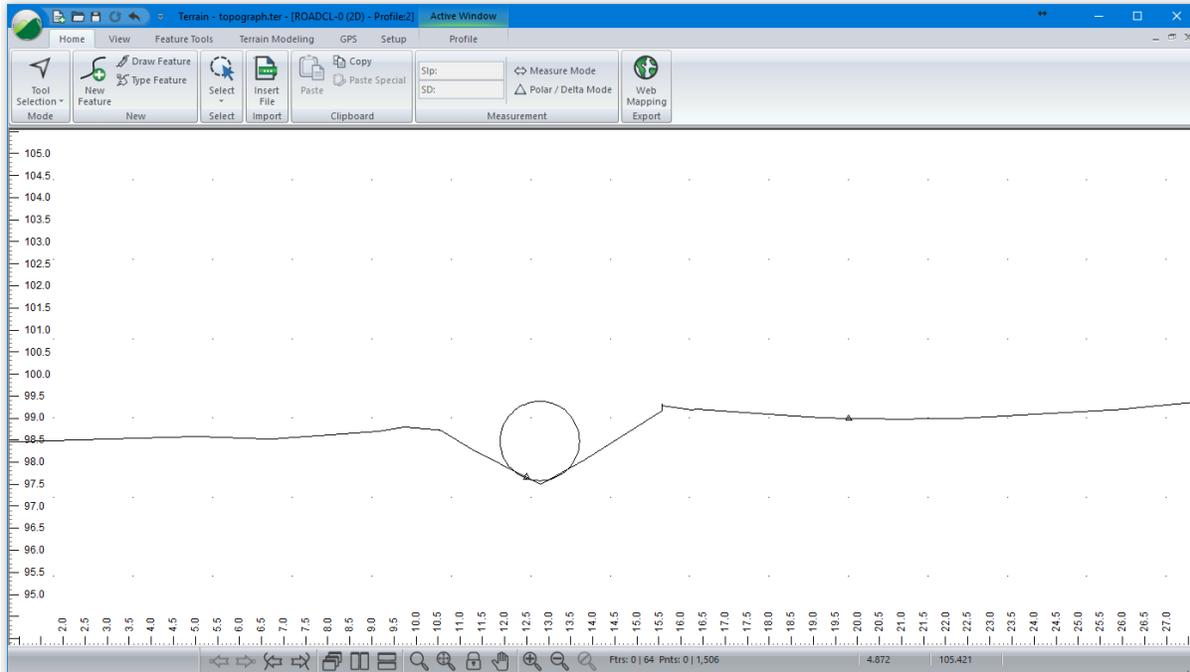
Figure 9-19: 1800 mm Pipe Displayed in Road Centerline Profile
