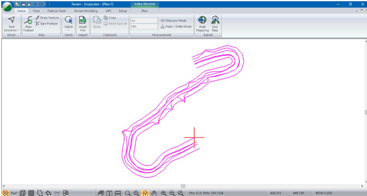
Figure 8-4: Imported Features (Road Edges, Slope Stakes and Right of Way)
