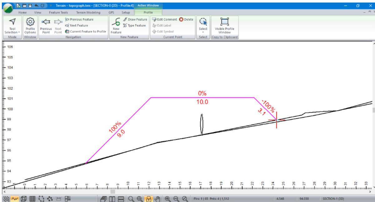
Figure 9-21: Cross Section with Road Template
