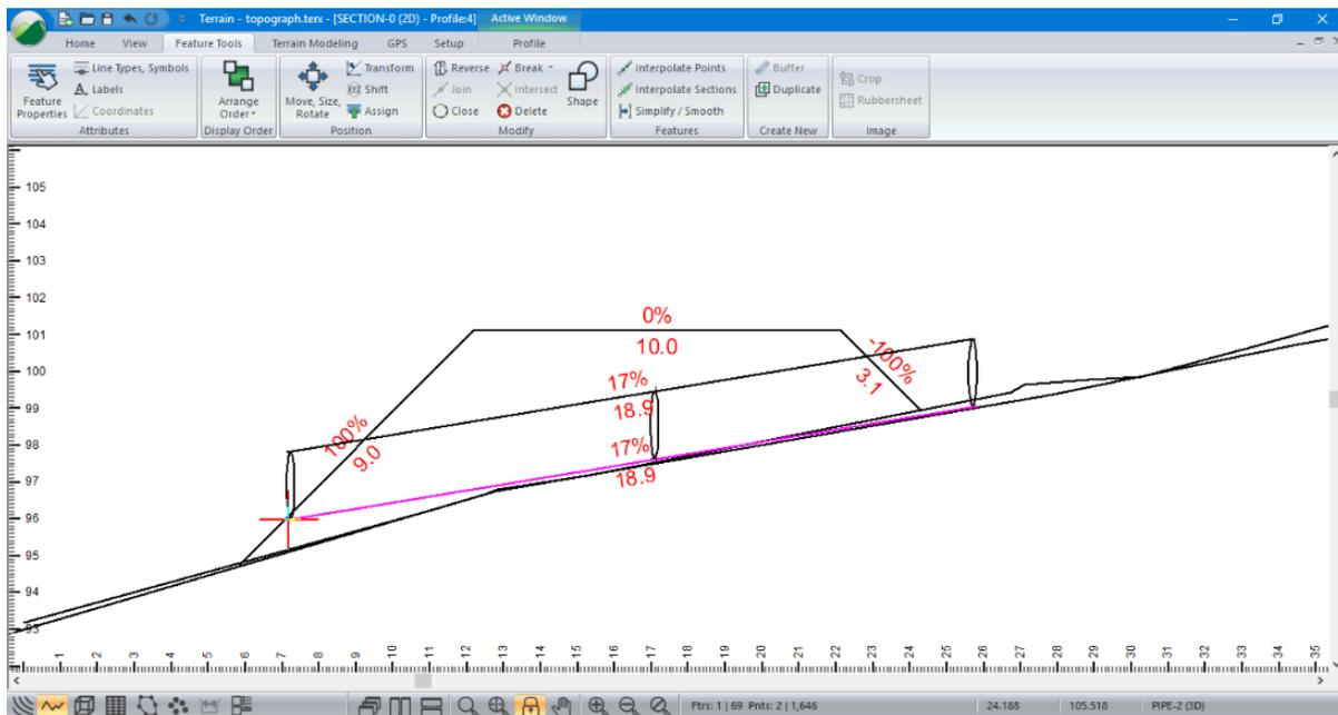
Figure 9-23: Cross Section with Culvert Position
