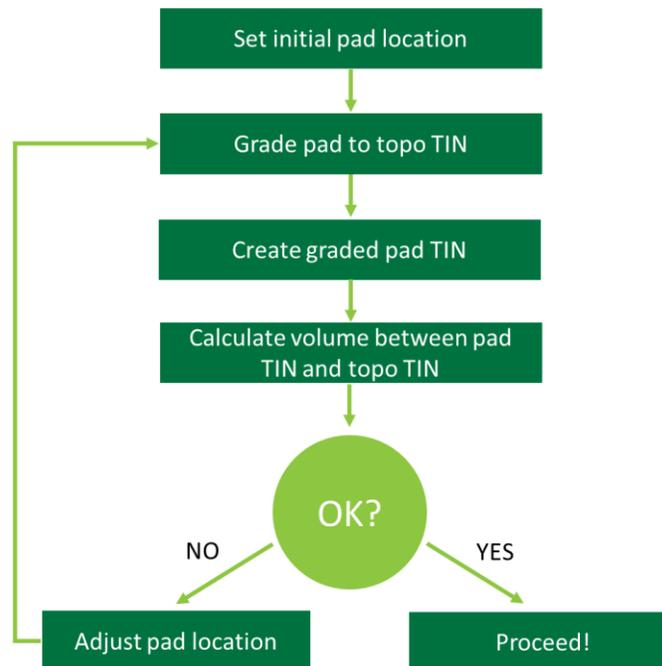
Figure 10-1: Procedure for Balancing Cut and Fill
