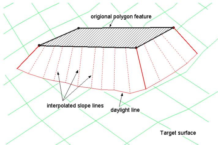
Figure 10-5: Grading a Polygon to a Target Surface
