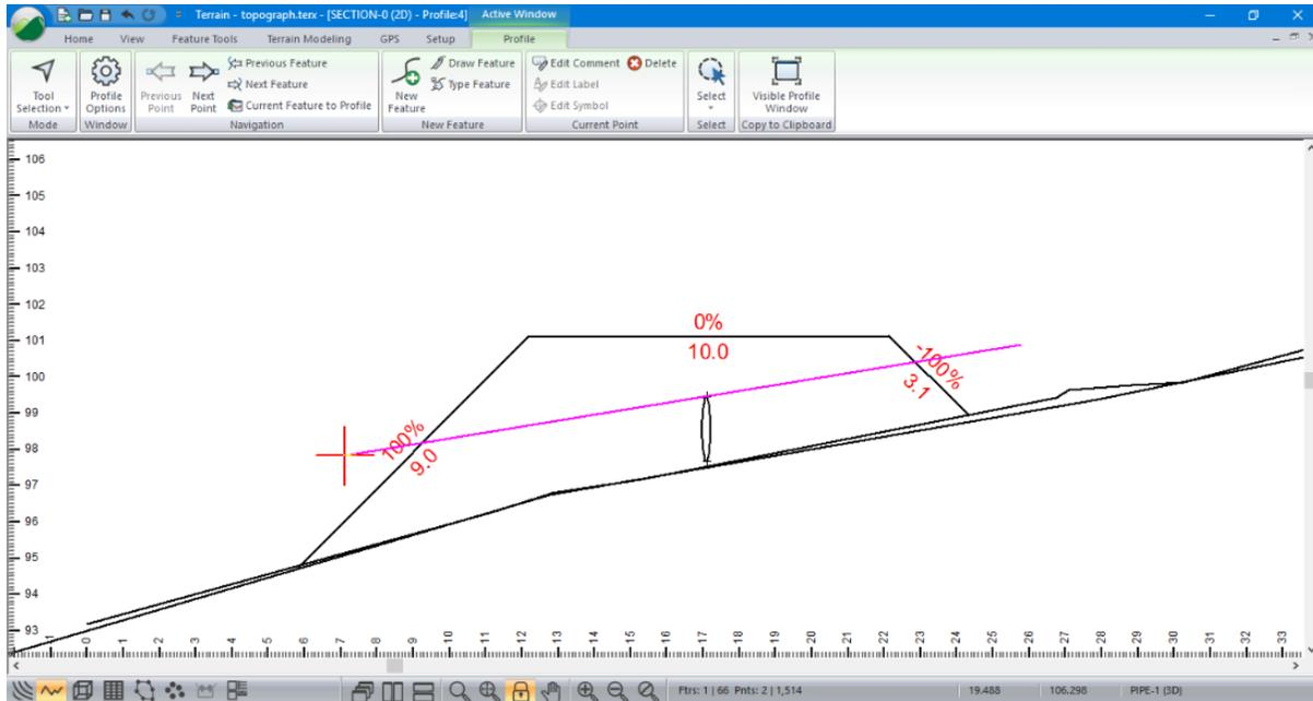
Figure 9-22: Cross Section with Preliminary Culvert Position
