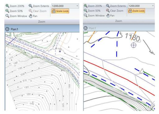
Figure 5-3: Zoom Out and Zoom In, Respectively, with Scale Locked
